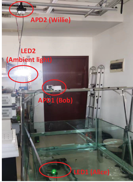
Fig. 13. The experimental system of W2A-OWC.
